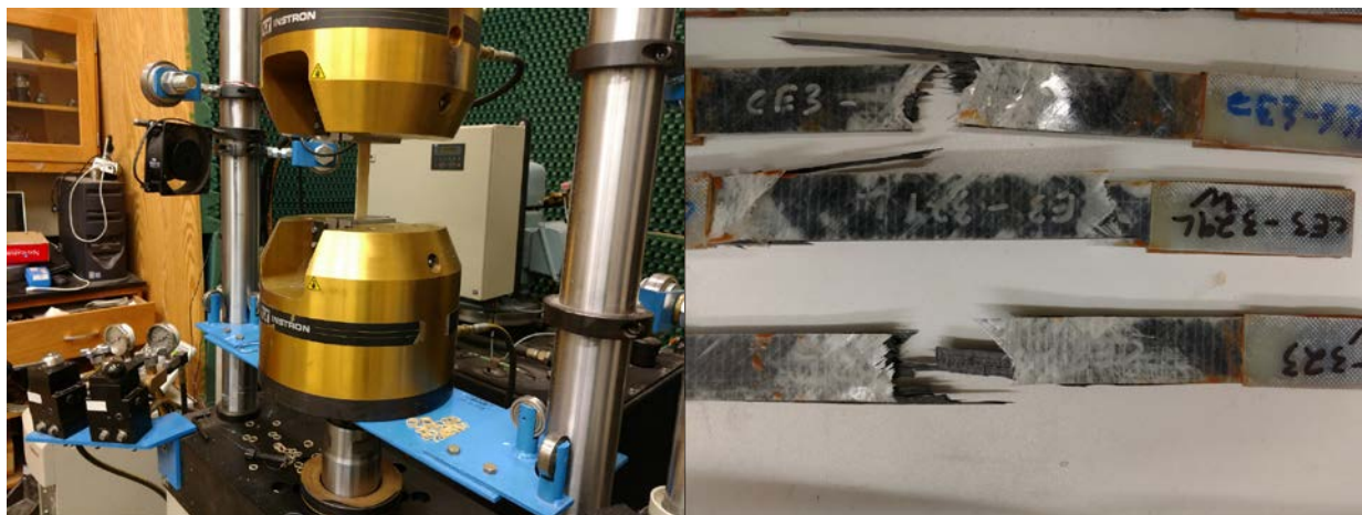
Figure 5. Coupon testing performed at Montana State University in BP1. Static and dynamic (fatigue) tension testing were performed as a preliminary evaluation of composite material sets in both dry and saturated (aged) states. Efforts in BP2 will focus on two material sets for comprehensive characterization of failure in accelerated life testing.
