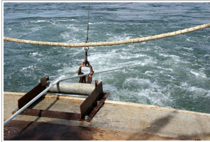
Figure 4. Anchor pull testing will be performed off a boat capable of deploying a 1 metric ton anchor, with instrumentation capable of determining pull loads for holding capacity estimates.
